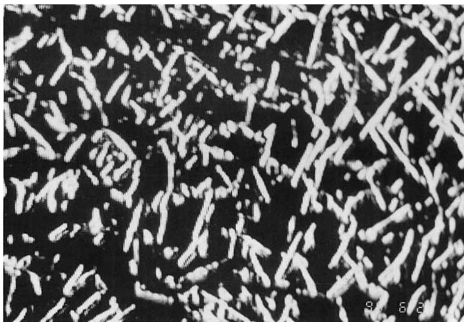
Figure 4 Polarizing optical micrographs of polymer, (A) PE2S3 at 177°C; (B) PE1S3KA at 145°C.
